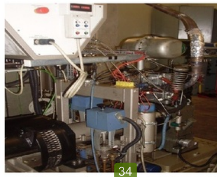
Figure 1. The installation of Hydra single cylinder diesel engine
